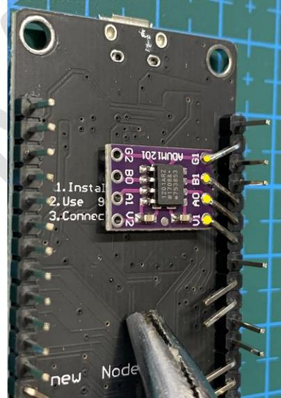
STEP 4A: **ONLY FOR JK** add Connection to GND and VCC Pin
